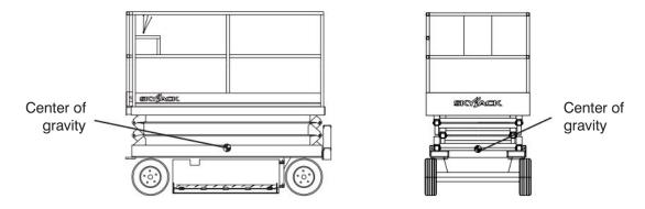
Figure 3-14. Center of Gravity
