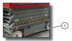
Figure 3-3. Pothole Protection Device
