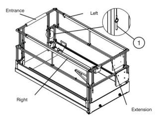
Figure 3-5. Folding Guardrail System
