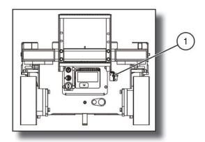
Figure 2-1. Main Power Disconnect Switch
