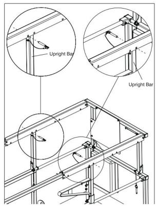
Figure 3-11. Variable Position Manual Extension
