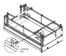
Figure 3-12c. All Guardrails Folded Down
