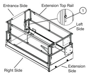
Figure 3-12a. Folding Guardrail System
